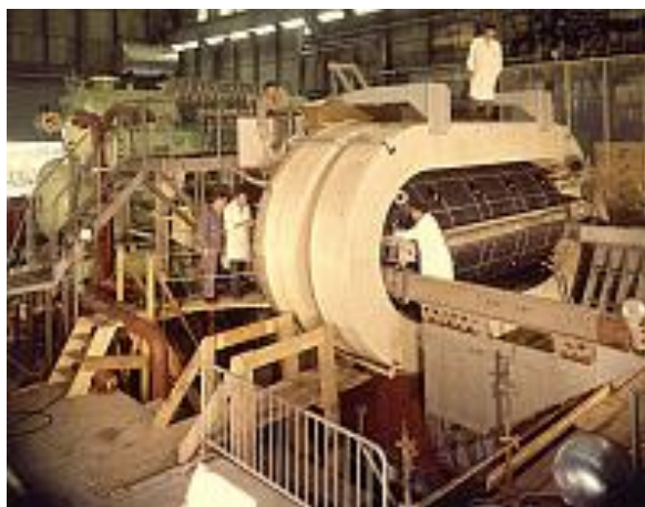
Gargamelle, the heavy-liquid bubble chamber at CERN in which neutral currents were discovered
